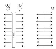
surface charge density for aluminum plate:
